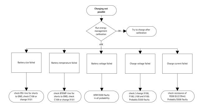
First thing you should do in case that charging of battery is not possible is to run energy management calibration. Note that calibration only works with JBV-1. In Service jig it is not possible because of missing bottom connector 1009.
