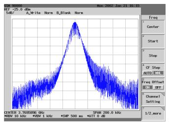
If no signal is measurable at T650 check VR7 2.6VDC at C650. If OK, set span of your analyser to e.g. 250MHz to check if the oscillator works on any other frequency as on the supposed. In case of that check control voltage at C652 which normally is 3VDC on channel 37. Especially check C653 (tendency to leak) in case of noise on the control voltage. In case that the oscillator does not work at all, change G650 and retest the phone.
