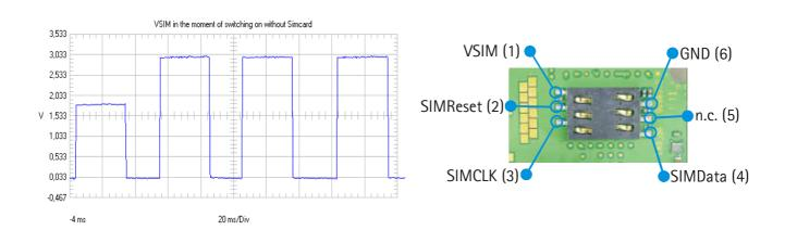
In case that the above mentioned signal is not measurable at one or more simlines, check SIM lines for shorts to ground. Resistance of simdata- and VSimline normally is  $> 200k\Omega$ , resistance of SIM reset- and SIM clock line normally is  $\sim 4.5M\Omega$ . If resistance of any line is not ok check parts the SIM lines consists of (R388, C203, C389).
